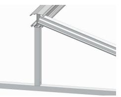
Make sure the glazing bar is in line with the gutter beam, then using the same fixing method as the wall plate secure the glazing bar to the gutter section. Your pre-drilled holes will determine where you drill through on the radius of the gutter section.
