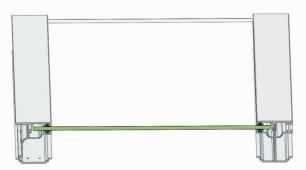
Cut the 'f'-section the same width as the distance between the inner edge of the two glazing bars. See the image below.
