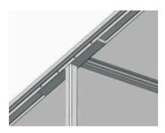
Image shows gutter channel fitted.
