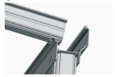
Repeat the above with the last glazing bar at the other end of the wall plate and gutter beam to stabilise the wall plate and gutter beam while you seal the wall plate in the following section.
